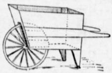
much less weight on the handles. The construction of the wheelbarrow is perfectly plain from the drawing. The box is three feet long, 21/2 feet wide into a little of the flour before addboards. The result was very satis-
