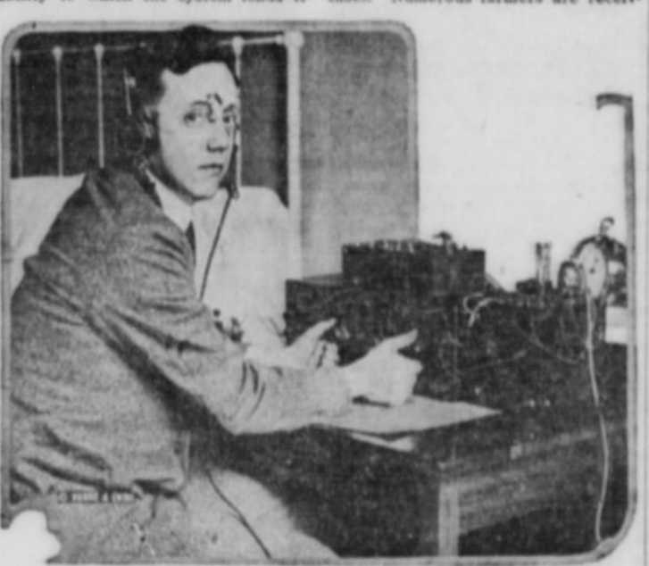
H. G. Corcoran of Washington, D. C., Needs No Aerial for His Radio Outfit, His Receiving Wire Being Connected to the Wire Springs of His Bed.
